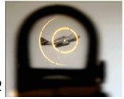
The principle behind a red dot sight is simple. The shooter views the target through a lens onto which a glowing dot and/or reticle is projected. If you've
