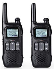
Family Radio Service (FRS) is very similar to GMRS, but it doesn't require a license. This feature means that the Radioddity FS-T1 FRS (pictured here) can be used right out of the box. All you need to do is ensure that you and the person on the other end are using the same channel.
