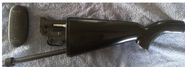
Charter Arms AR-7 broken down for buttstock storage
