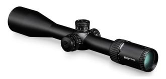
It is constructed of 30MM machined aircraft-grade aluminum that is filled with nitrogen and sealed with O-rings to combat the scope from fogging over or taking on water. It measures in at 14.9 inches and weighs 25.6 ounces. Due to its thickness, the internal adjustment range is increased, which, when coupled with the magnification range, makes shooting at targets near and far a breeze.
