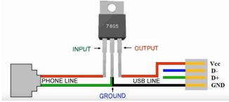
Because the power is out, you'll likely need to wrap the exposed wires around the indicated areas. Be sure they're wrapped away from each other. Plug your phone into its cord, then plug the cord into the USB connection. It should begin to charge your phone, and you'll have enough battery within a few minutes to make a phone call.
